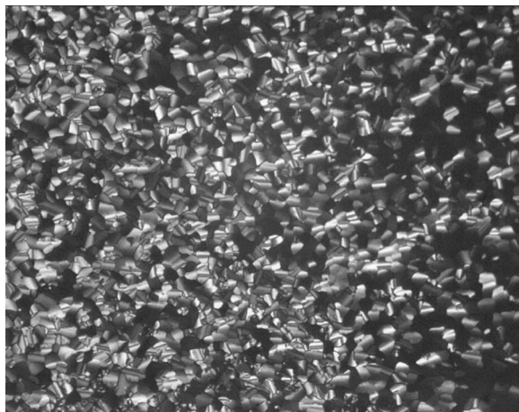
FIGURE 3 Texture of 9b obtained with a polarizing microscope on cooling at 100°C ( \times 200 )
